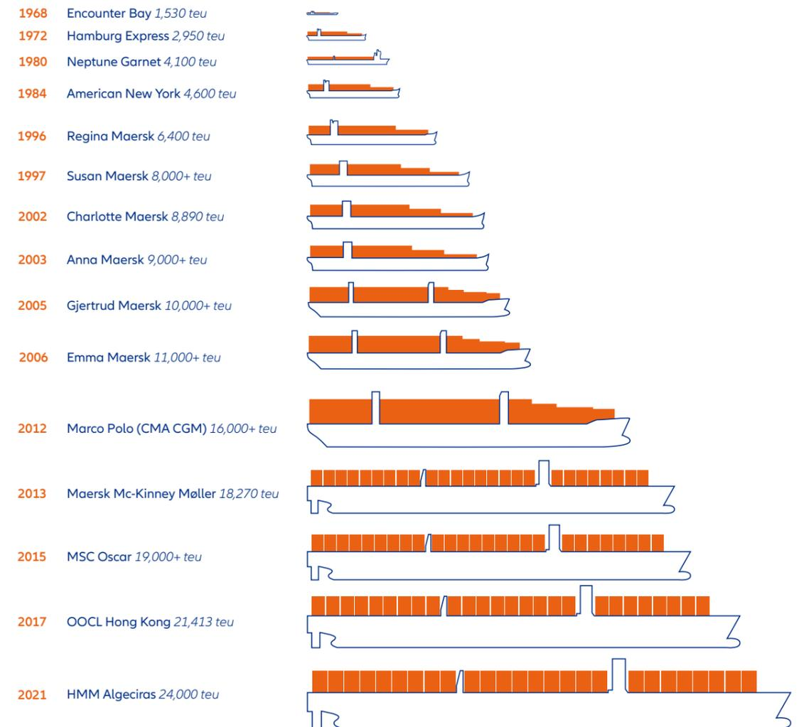
Container-carrying capacity has increased by around 1,500% since 1968 and has almost doubled over the past decade. Ever larger vessels are on order.
